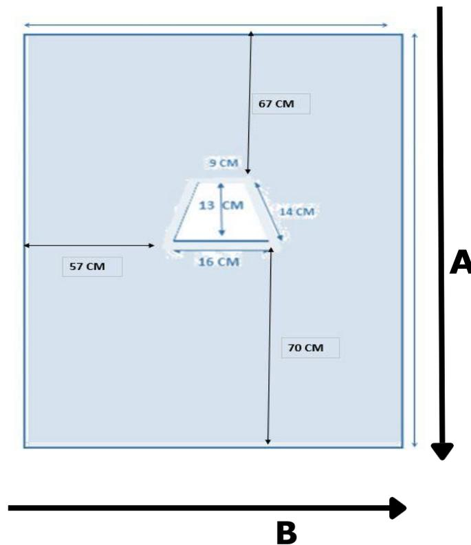
**Figure 1.** O.P.U Drape Technical Specifications
